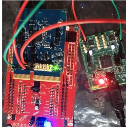
**Figure 12. HCI TX/RX Sniff With CC2564xQFN-EM Module**
