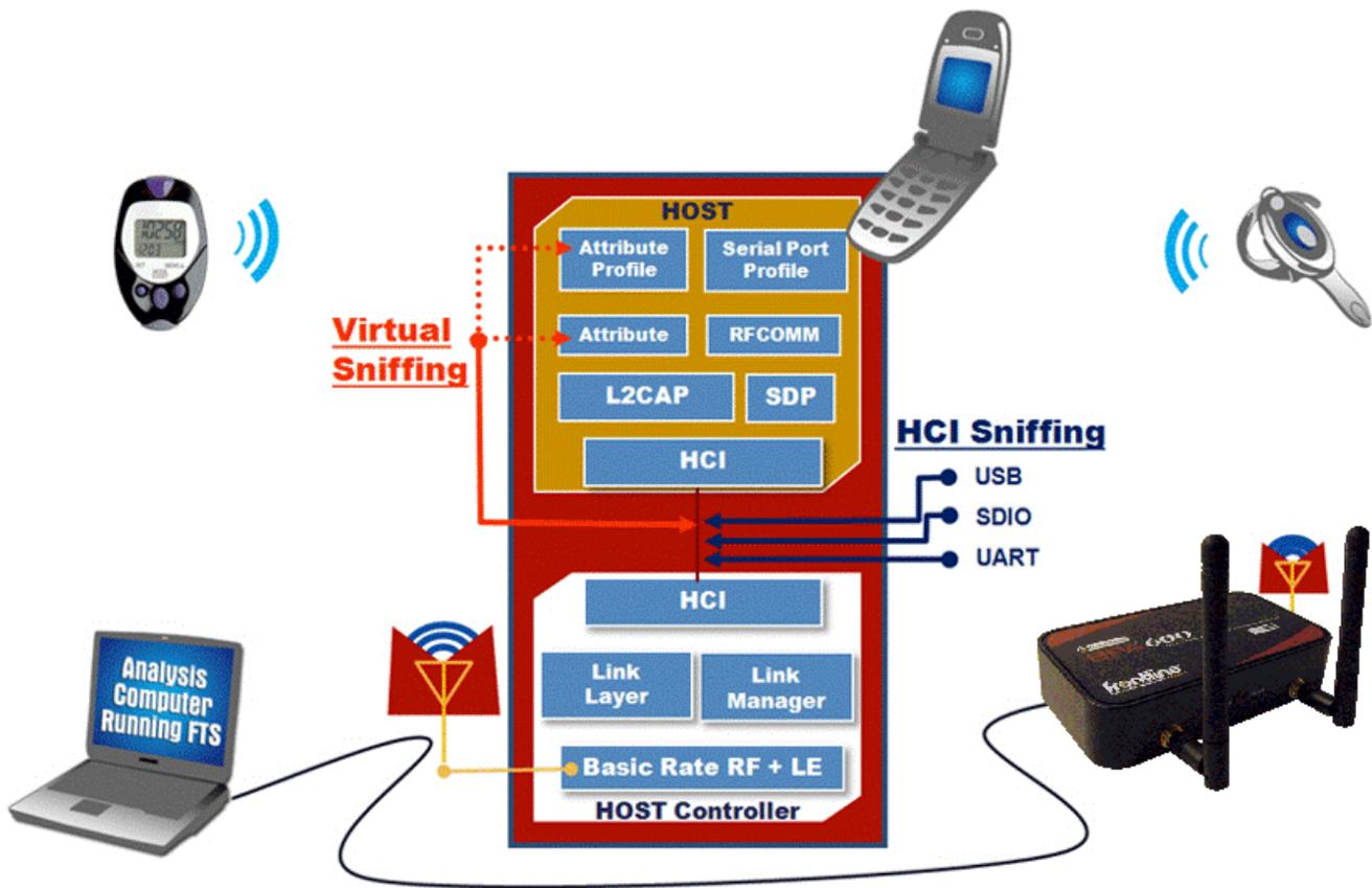
Figure 10. Frontline Technologies HCI Sniffer (Using Serial Sniffer)
