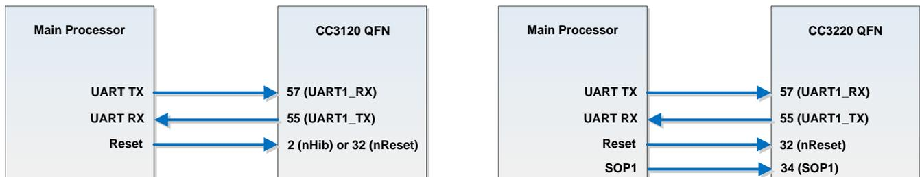
**Figure 1. CC3120 and CC3220 QFN Programming Setup**
