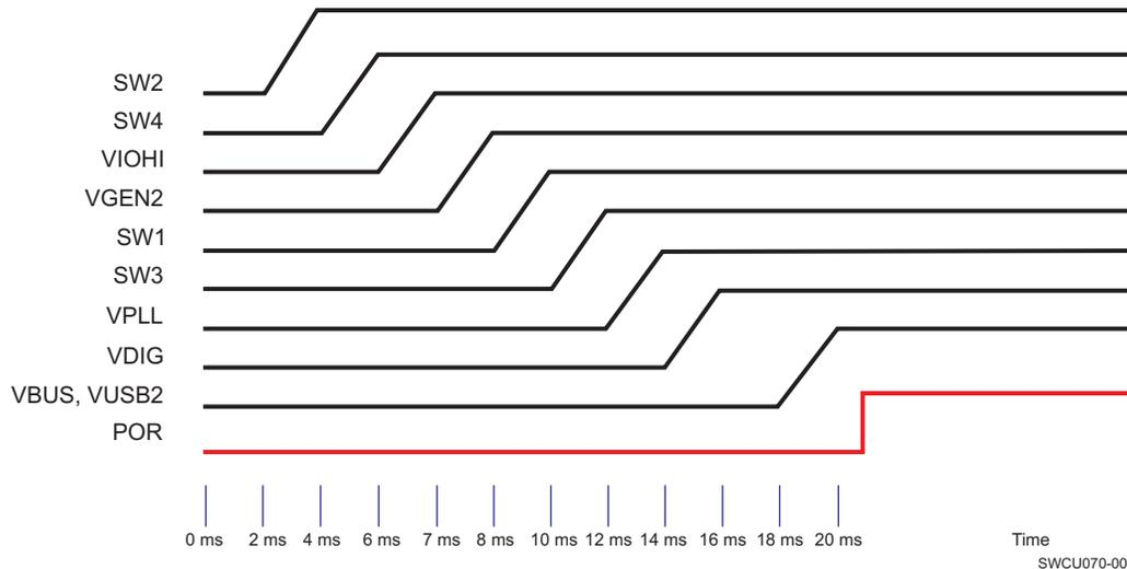
Figure 4. Timing Diagram of Power Rails for MC13982 (Source: Freescale AN4053.pdf Application Note)
