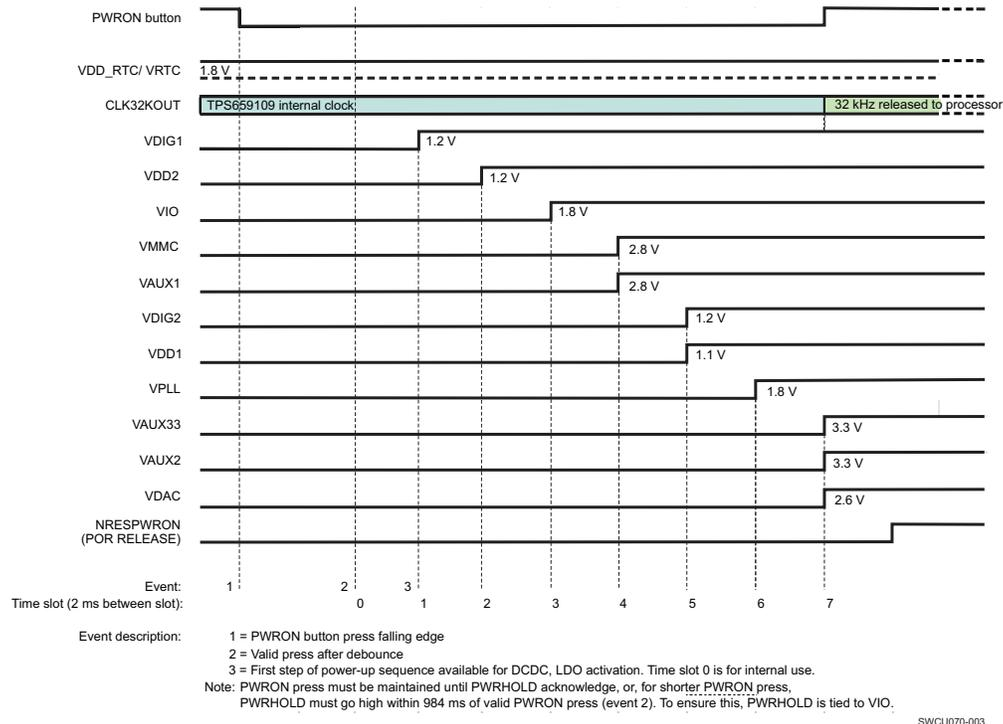
Figure 3. Power-Up Timing Diagram
