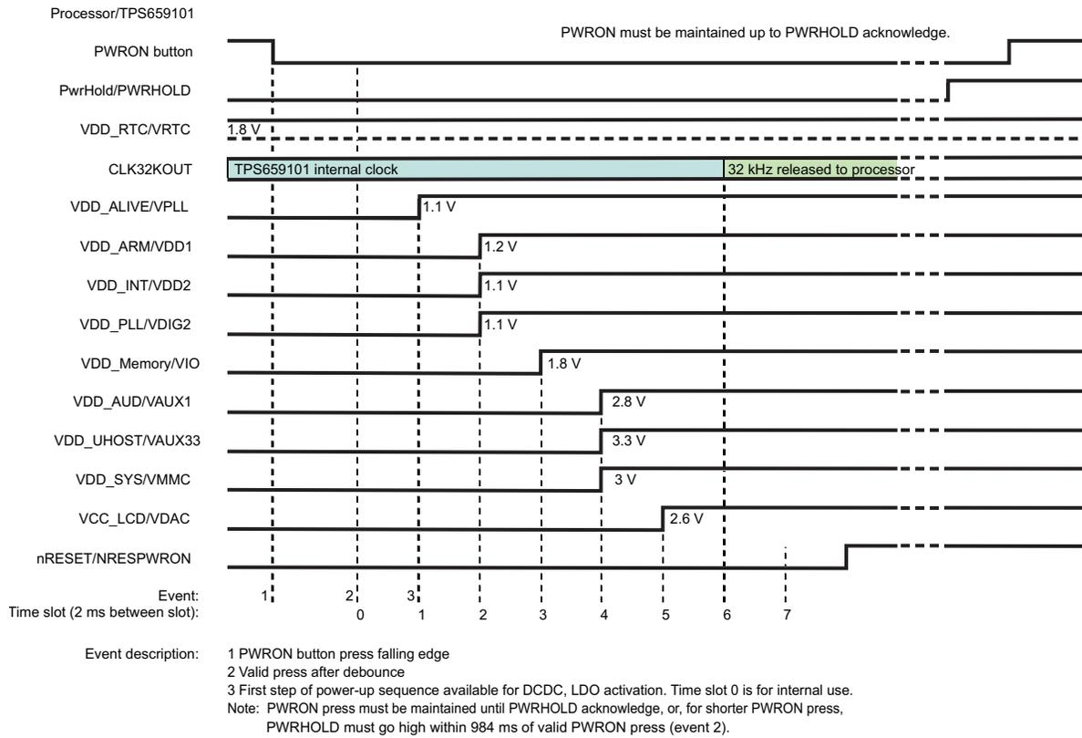
Figure 2. Power-Up Sequence Programmed on TPS659101 EEPROM
