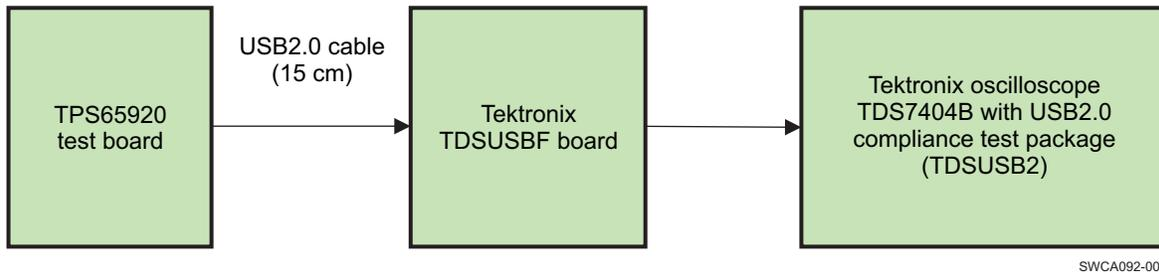
Figure 4. USB Eye Diagram Setup
