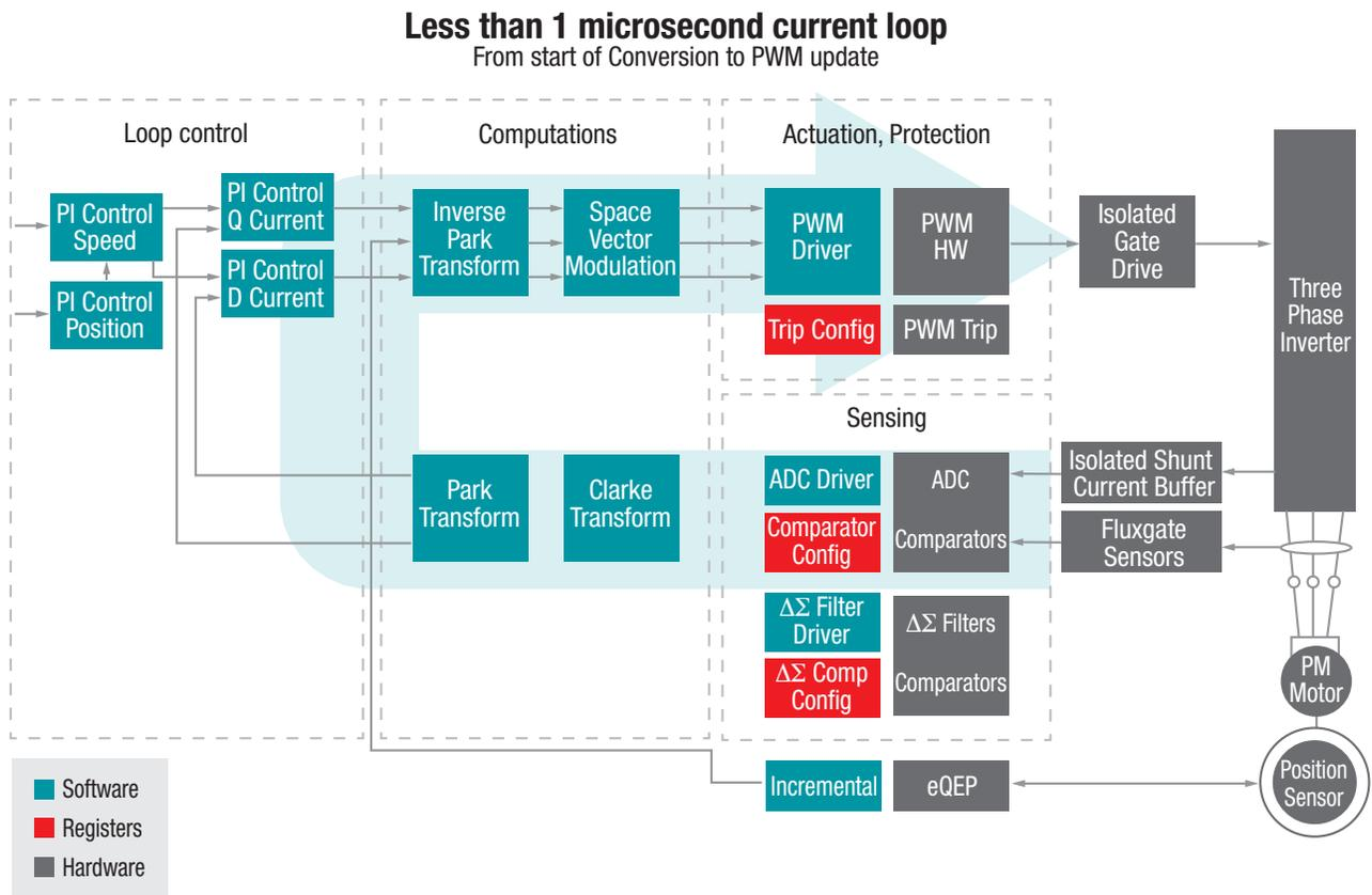
Figure 1. Less than 1  $\mu$ s current loop with FCL (replace “QEP” with “Resolver” in the picture).
