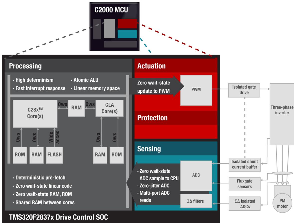
Figure 3. C2000 MCU architecture for real-time motor control
