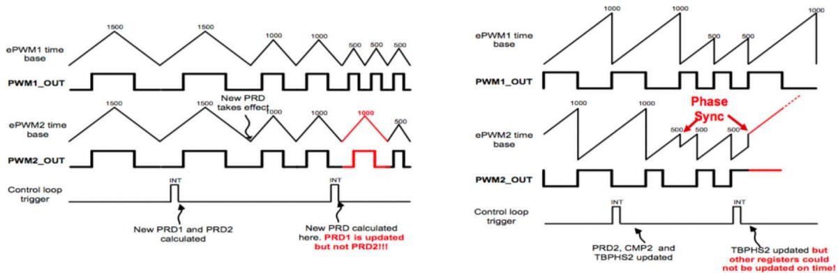
Figure 11. Challenges for variable-frequency PWM waveform generation.
