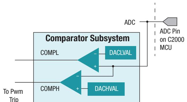
Figure 6. The CMPSS used for overcurrent protection.
