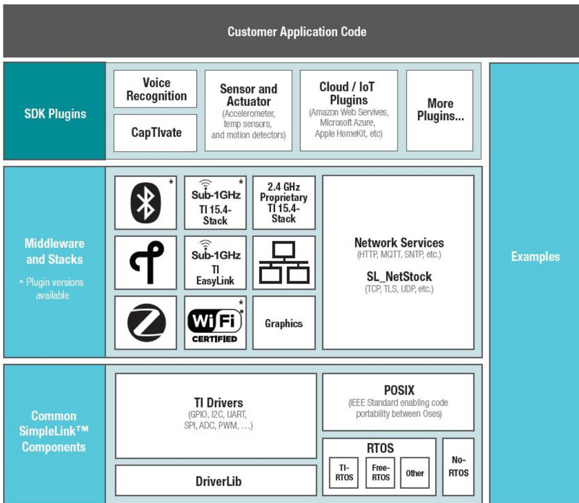
Figure 3. SimpleLink SDK diagram.
