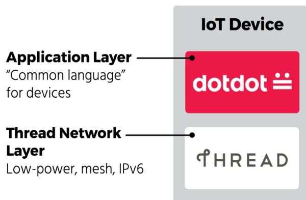
**Figure 2:** Thread and Dotdot application layer.
