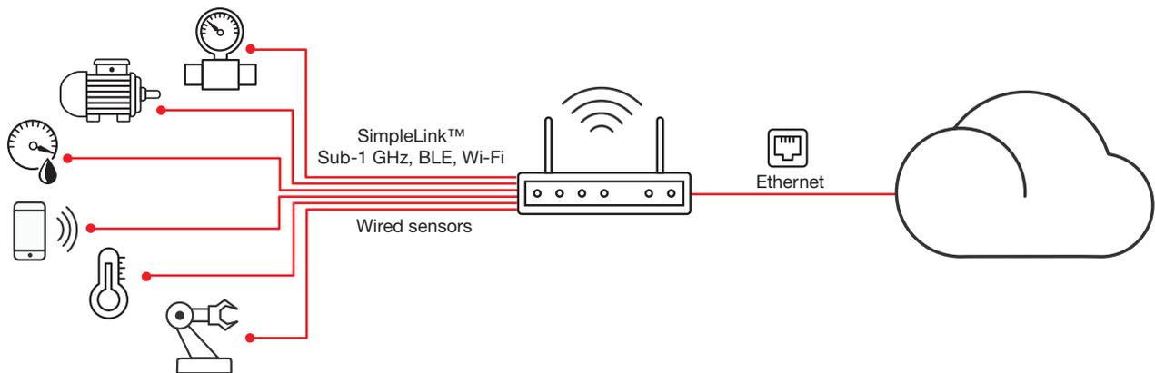
**Figure 3.** SimpleLink MSP432E4 MCUs are the industry's most integrated Arm® Cortex®-M4 MCUs, with an integrated 10/100 media access controller plus physical layer (MAC+PHY) for implementing intelligent gateways.
