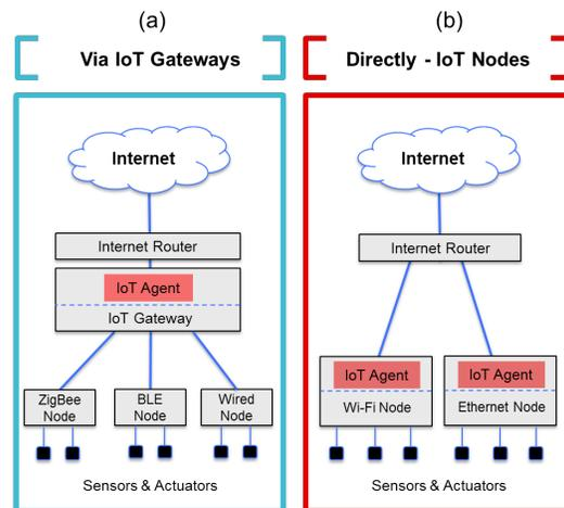
**Figure 2.** An IoT gateway can simplify connectivity design for sensor nodes by centralizing IoT functionality in the gateway. Nodes connect to the IoT via a gateway using both wired and wireless technology (a); nodes connect directly to the internet using a WAN connection such as Wi-Fi or Ethernet (b).
