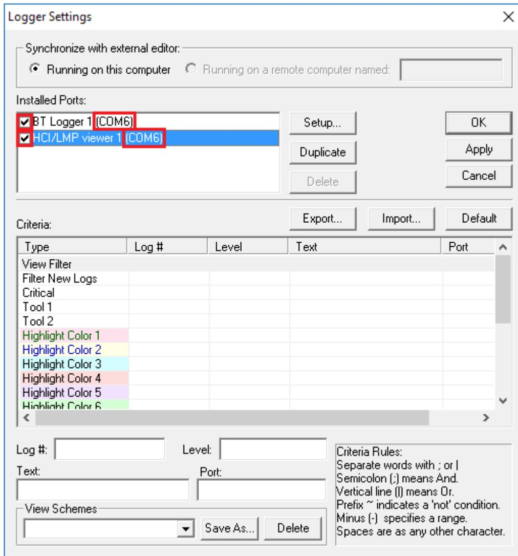
Figure 13. Properly Configured Logger Settings
