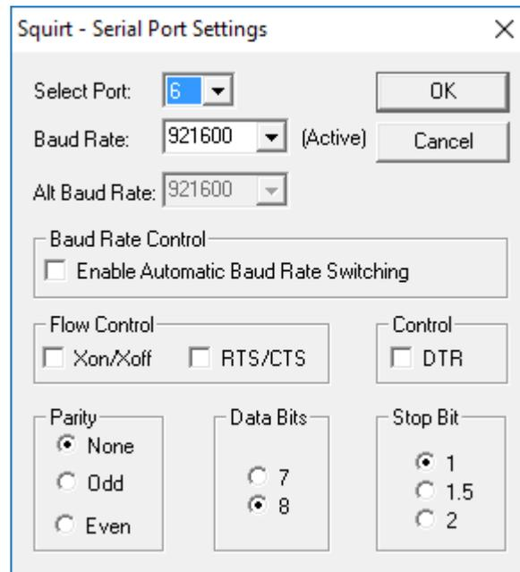
**Figure 11. HCI/LMP Viewer Serial Port Settings**
