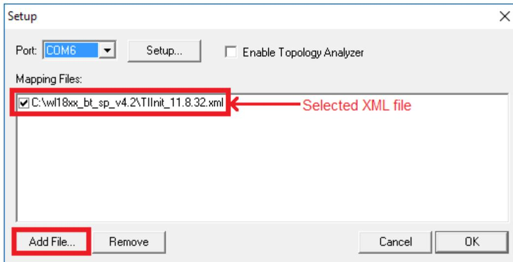
**Figure 12. Adding the XML File**
