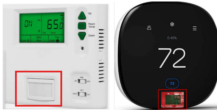
Figure 3-2. PIR size vs mmWave Radar Size in Thermostat
