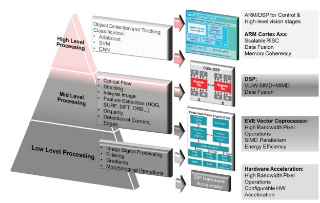
Figure 6. TDA2x SoC heterogeneous architecture.
