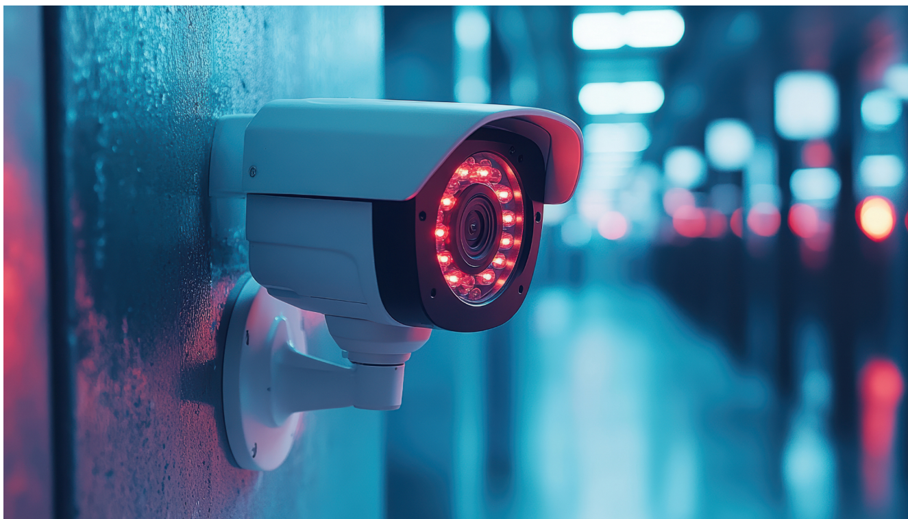
Figure 1. An Internet Protocol network camera using ambient light sensors and infrared LEDs
