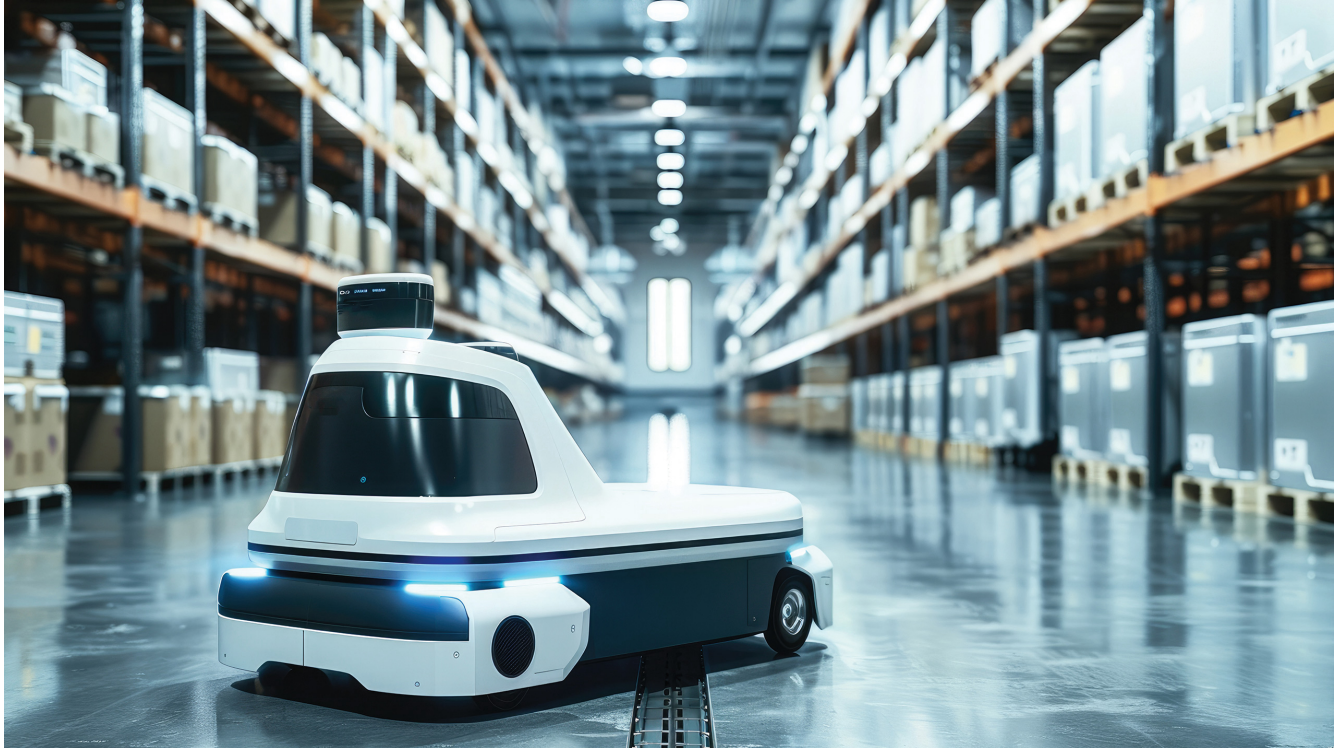
Figure 1. An AMR using lidar to navigate
