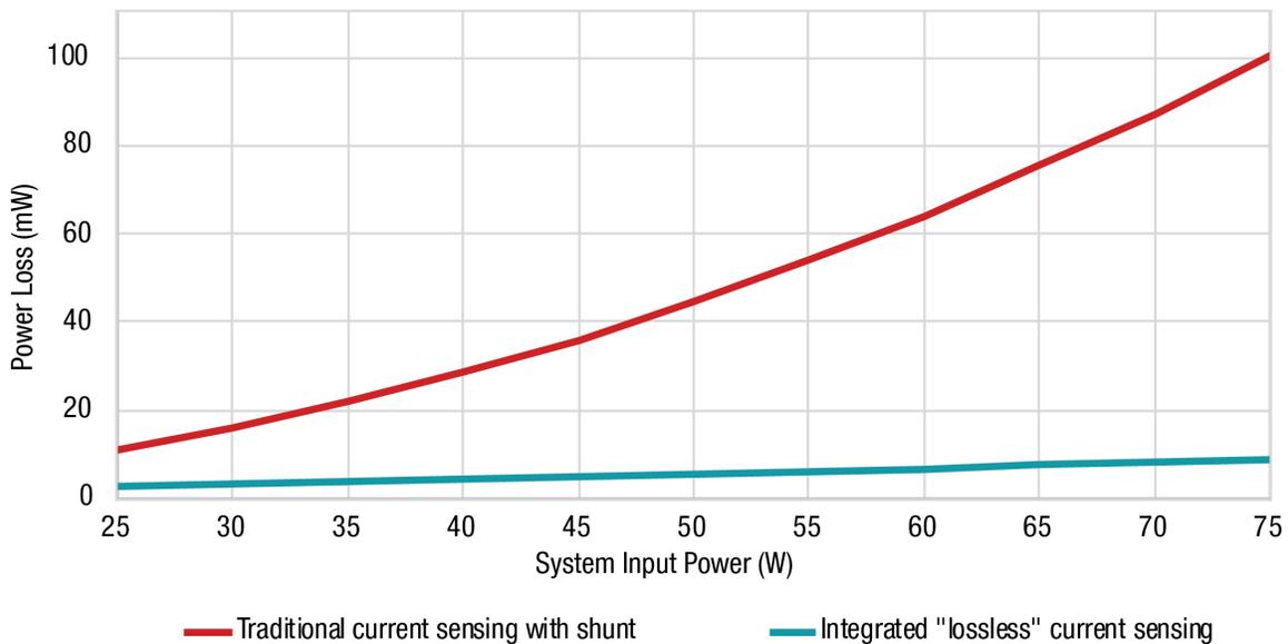
Figure 2. Integrated current sensing vs traditional current sensing power loss
