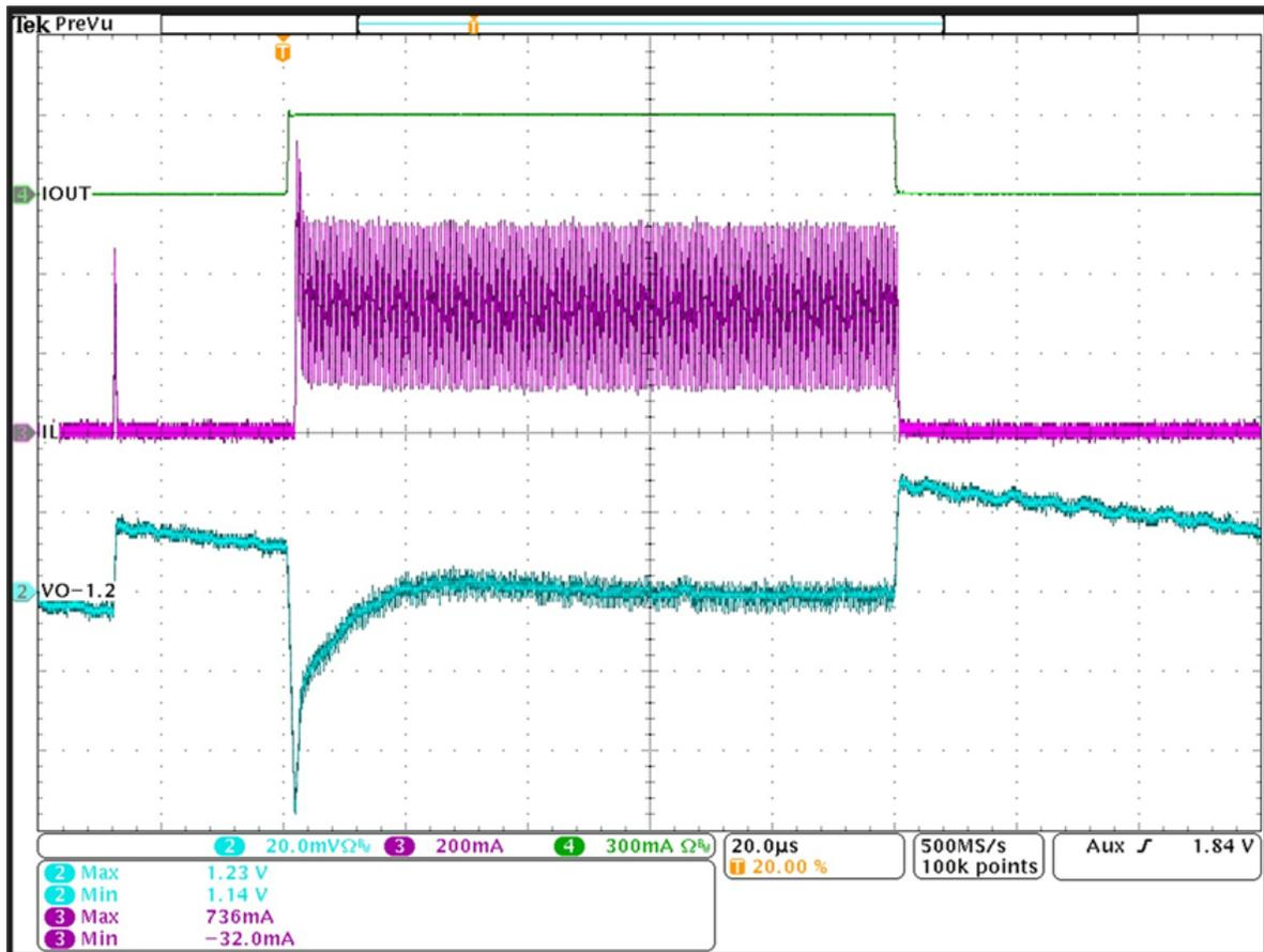
Figure 1-2. The **TPS62843** load transient at 1.2 V<sub>OUT</sub>, I<sub>OUT\_MIN</sub> = 0 A to I<sub>OUT\_MAX</sub> = 300 mA
