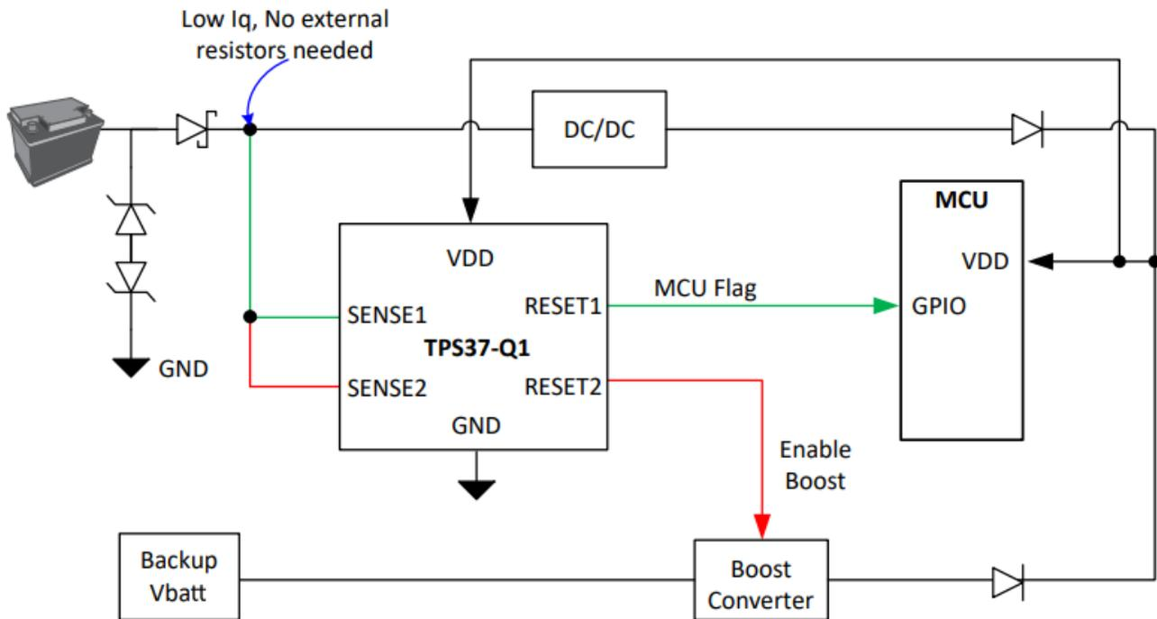
**Figure 1-1. Direct 12-V/48-V off-battery voltage monitoring with [TPS37-Q1](#)**
