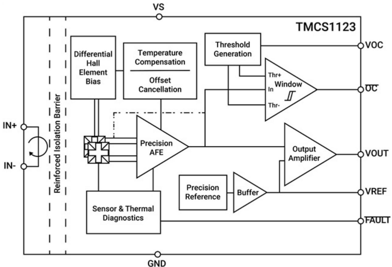
Figure 1-1. TMCS1123 block diagram
