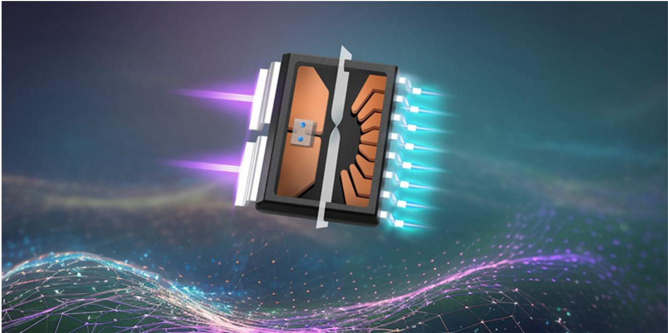
In electric vehicle (EV) charging and solar inverter systems, current sensors measure current flow by monitoring the voltage drop across a shunt resistor or the magnetic fields generated by current flowing through a conductor. These high-voltage systems use current flow information to control and monitor power conversion, charging and discharging.
