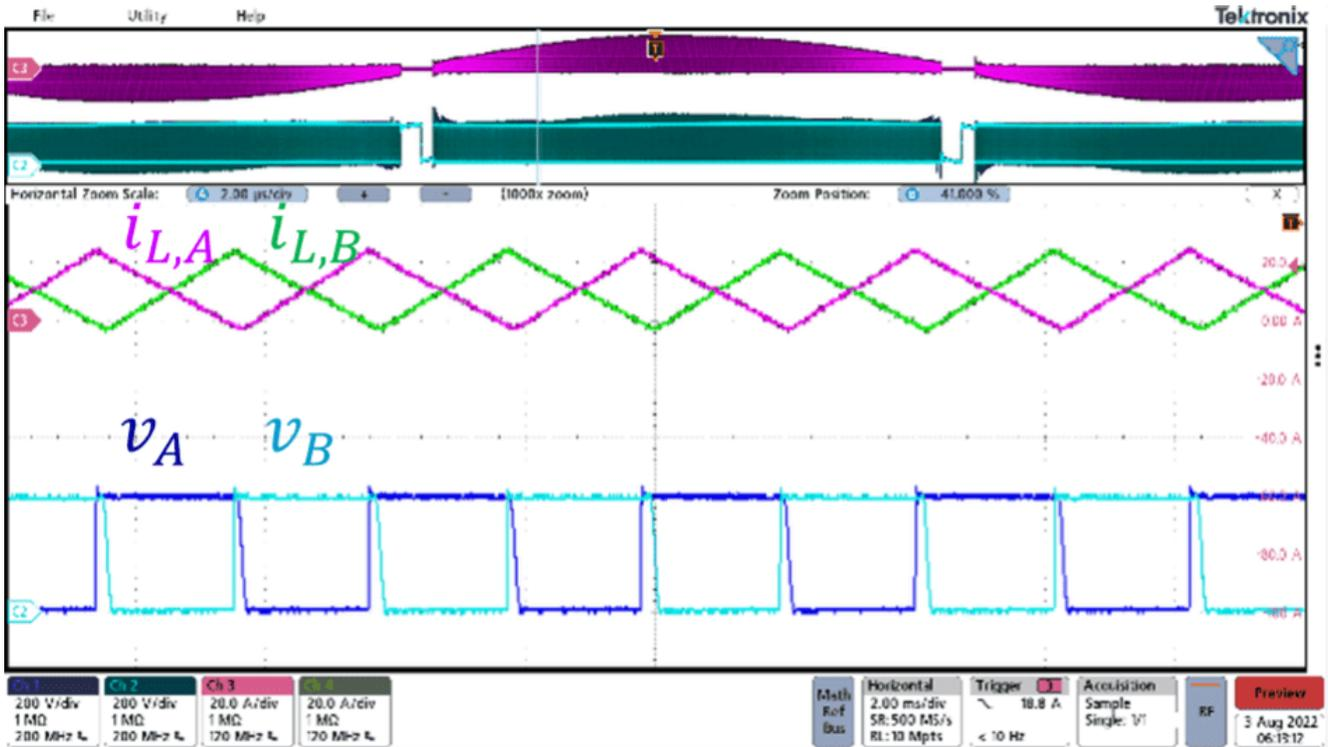
Figure 6. System waveforms of the prototype operating under full power ( $V_{in} = V_{out}/2$ , load = 5 kW,  $V_{in} = 230 V_{ac}$ ,  $V_{out} = 400 V$ ).
