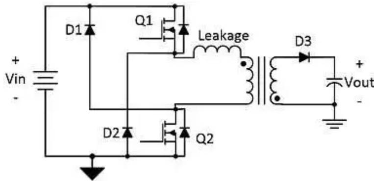
**Figure 2. The two-switch flyback recycles leakage energy to the input.**
