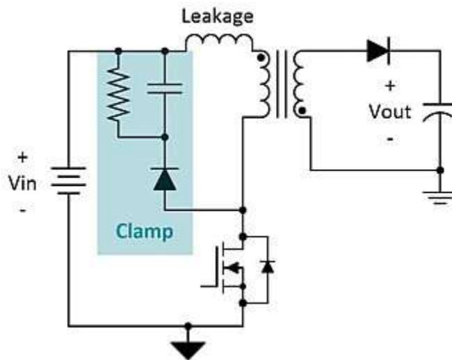
**Figure 1. Most flyback converters employ a dissipative clamp.**
