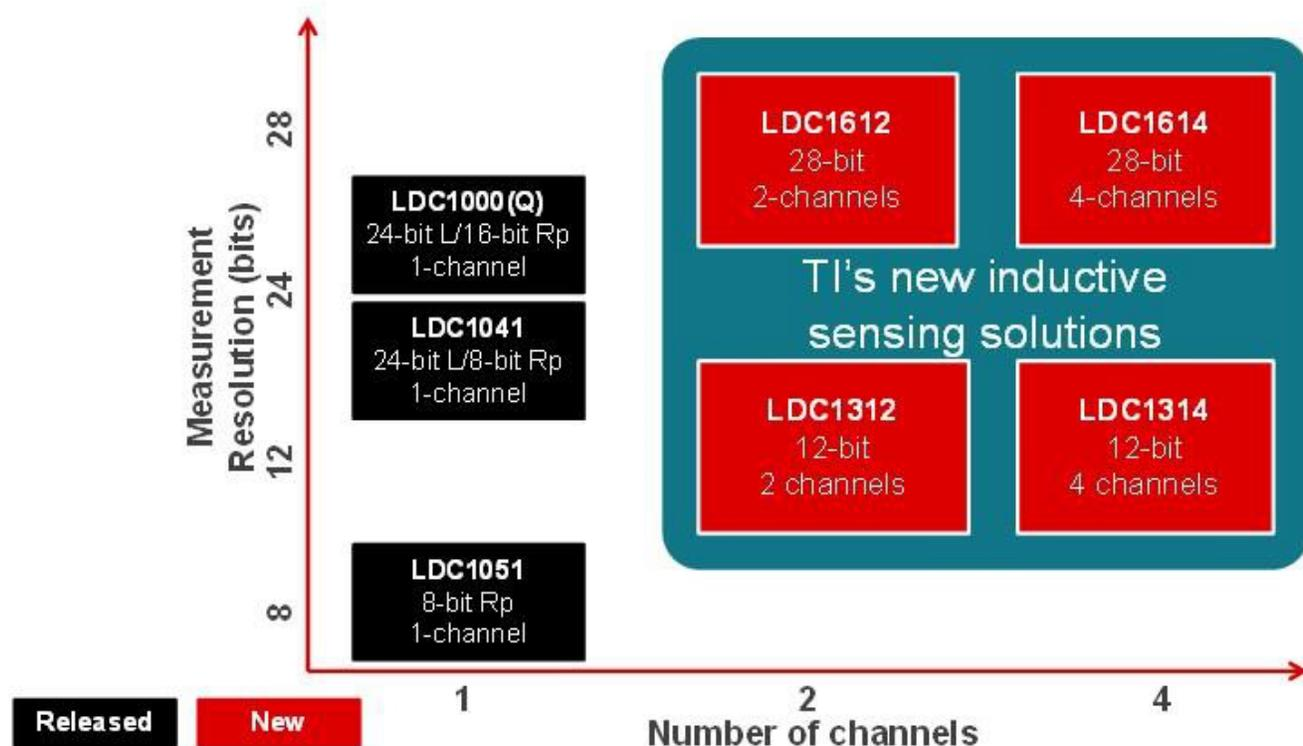
Figure 1. TI's New Inductive Sensing Solutions
