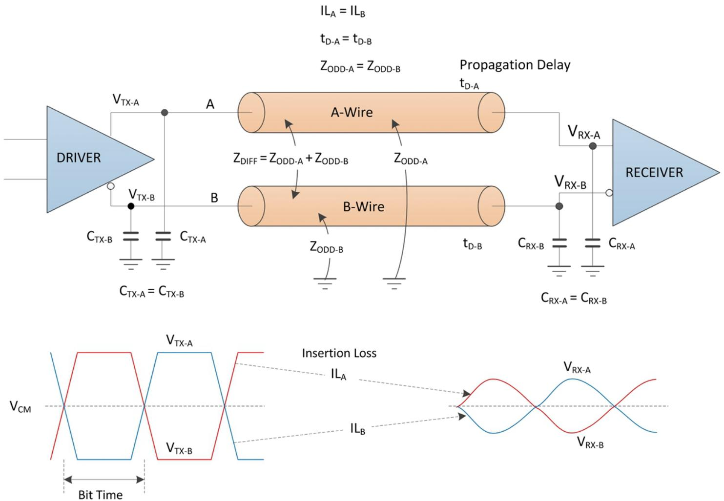
Figure 1. Electrical Properties for a Perfect Differential Pair
