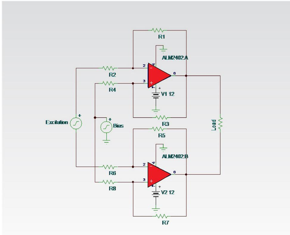
**Figure 2. Excitation Coil Drive Using the [ALM2402-Q1](#)**
