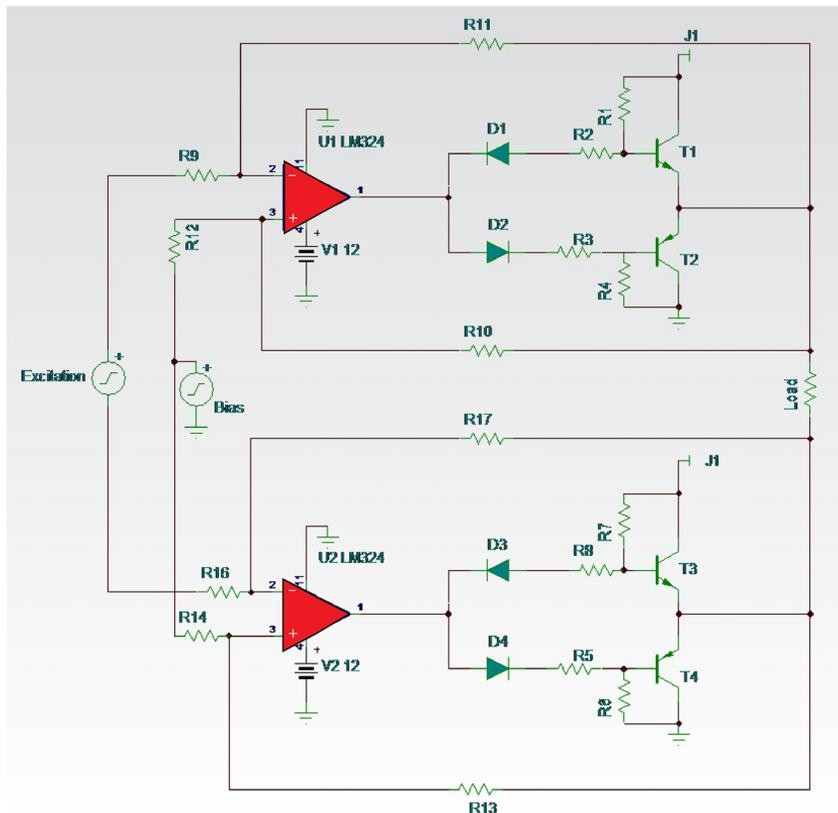
Figure 1. Discrete Implementation of Driving an Excitation Coil
