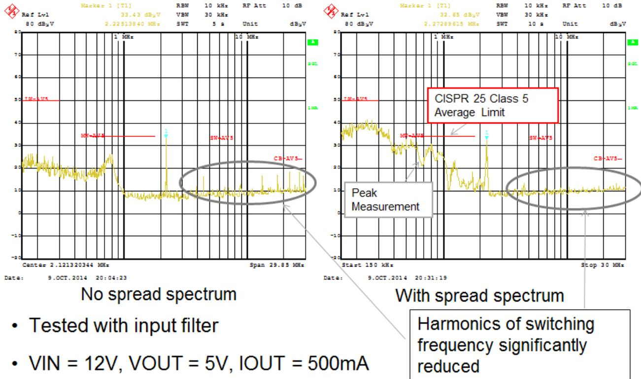
**Figure 1. Conducted Band CISPR 25, Class 5 with and without Spread Spectrum**
