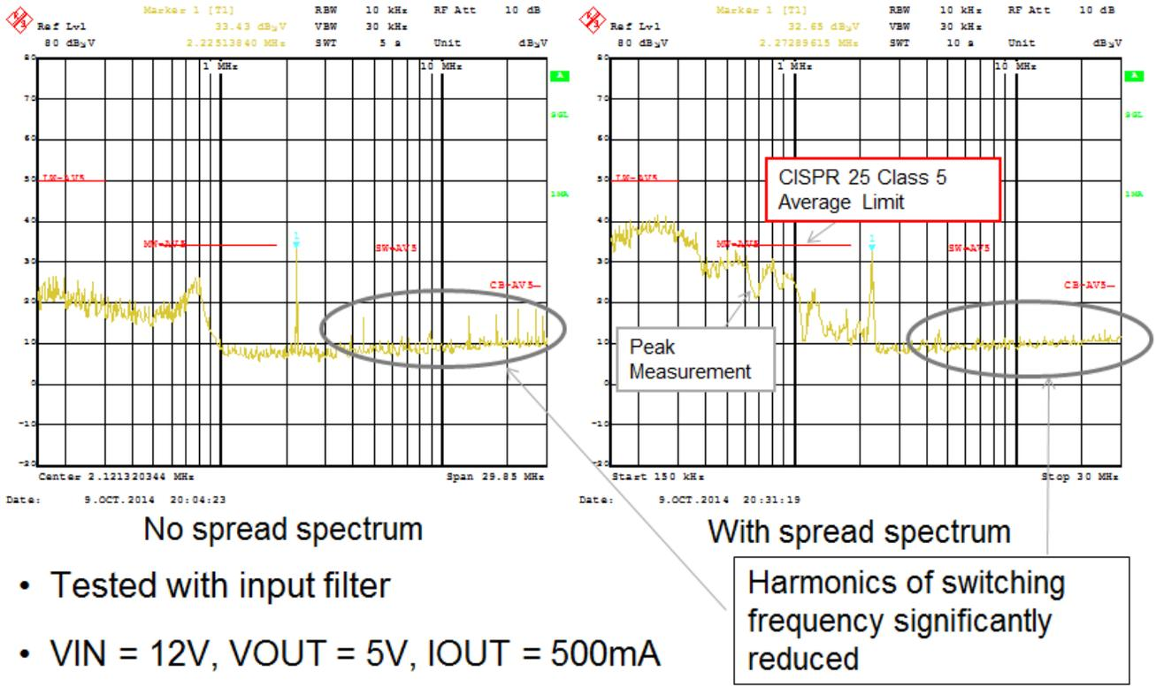
Figure 2. PMP9458 Reference Design for the LM26003-q1 And LM26420-q1
