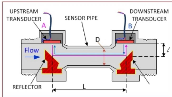
Figure 1. Ultrasonic Sensor Cell
