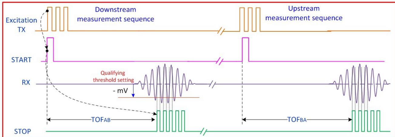
**Figure 2. Upstream and Downstream Transmit-Receive Sequence for Measurement of Difference in TOF**
