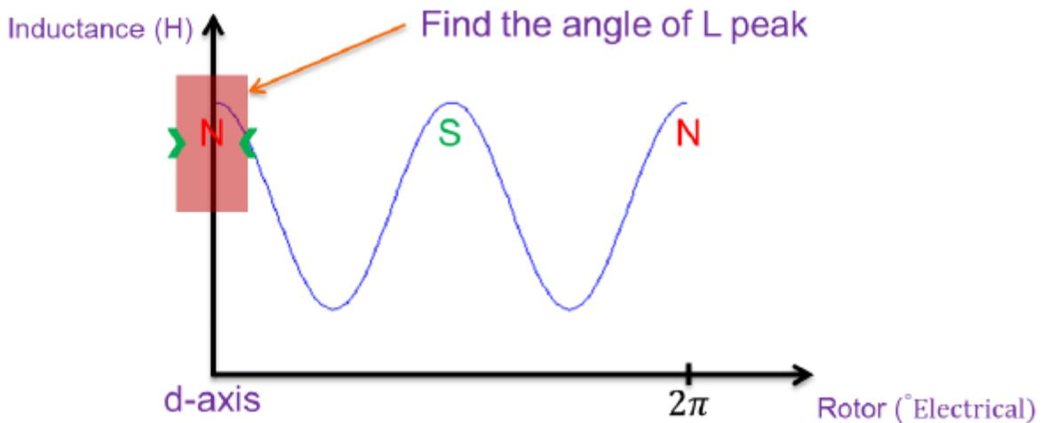
**Figure 4. Inductance variation of a highly salient rotor**
