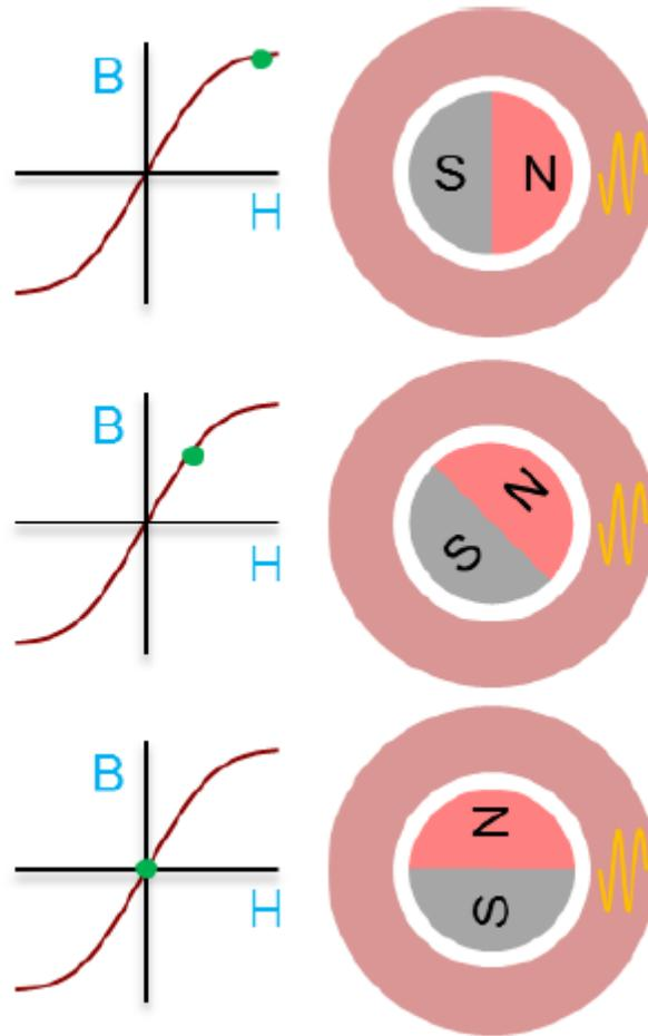
**Figure 2. BH curve and relative location for different rotor orientations**
