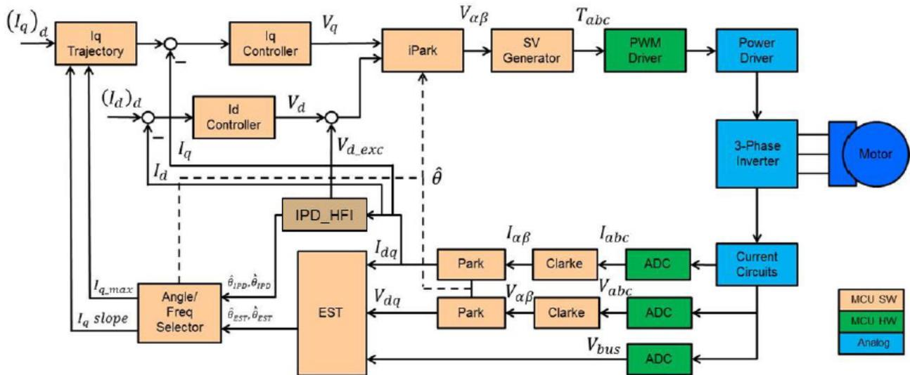
Figure 5. InstaSPIN-FOC with FAST (EST), IPD\_HFI, and AFSEL
