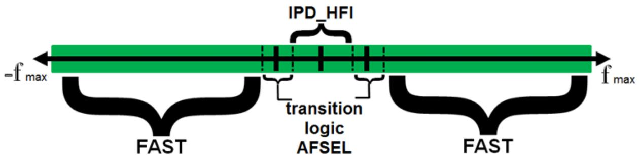
Figure 1. Frequency of operation with FAST and IPD\_HFI
