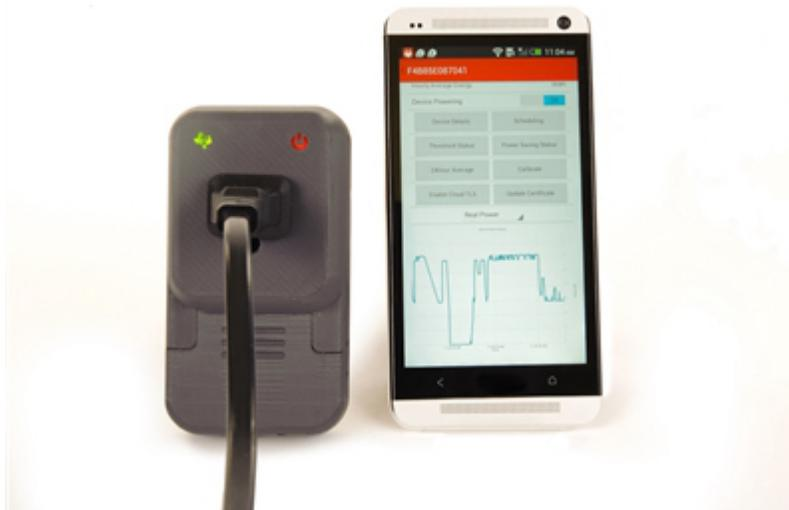
The SimpleLink Wi-Fi CC3200 Smart Plug monitors real-time energy consumption and records long-term energy trends, making way for financial returns through energy savings. It enables the Internet of Things (IoT) by bringing the ability to control and monitor electronics and multiple outlets remotely. Below are a few example applications that may spur inspiration to start designing your own smart plug with the help of our TI Design reference design.
