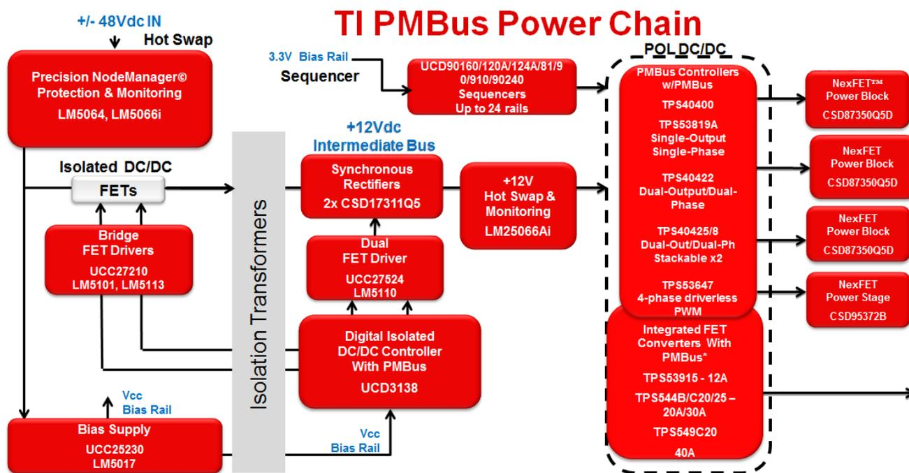
Figure 1. TI's PMBus Power Chain Diagram.
