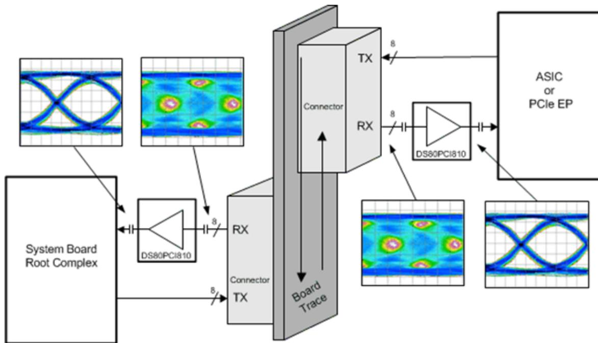
**Figure 1. DS80PCI810 PCIe Gen 3 Redriver Typical Application Block Diagram**
