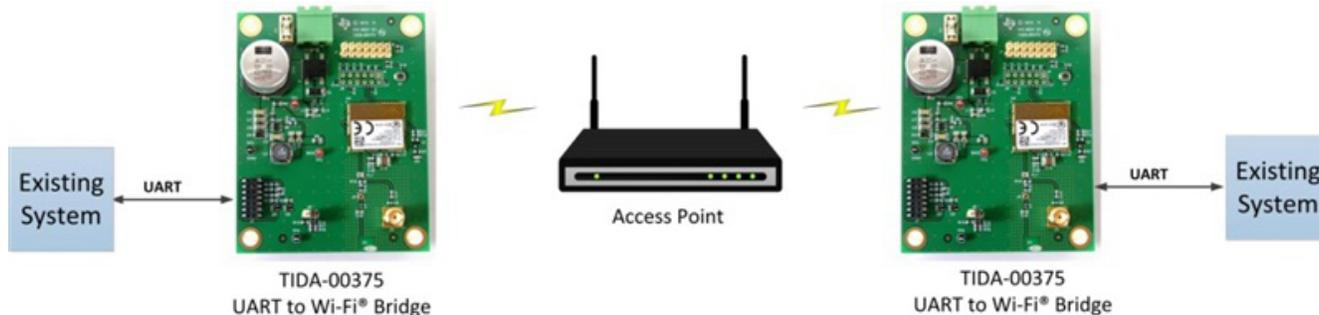
**Figure 1. Wireless bridge over an existing Wi-Fi network**
