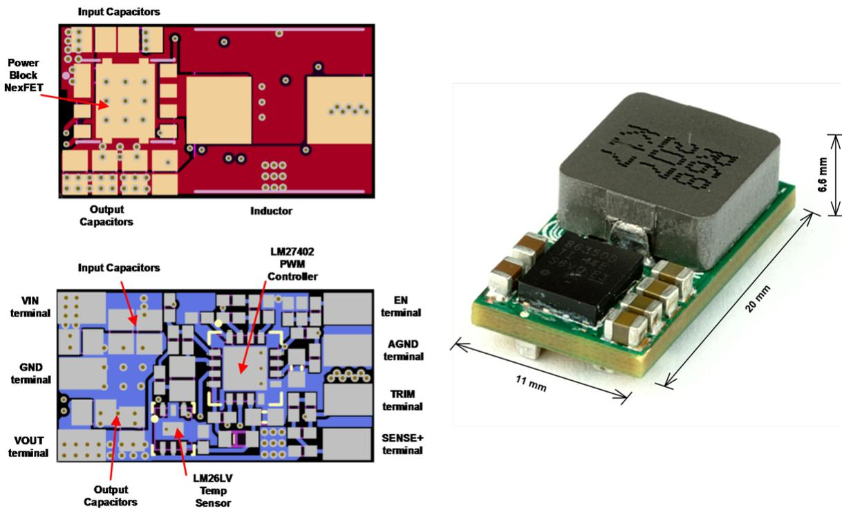
**Figure 1. 25A Synchronous Buck Converter PCB Layout and Implementation.**
