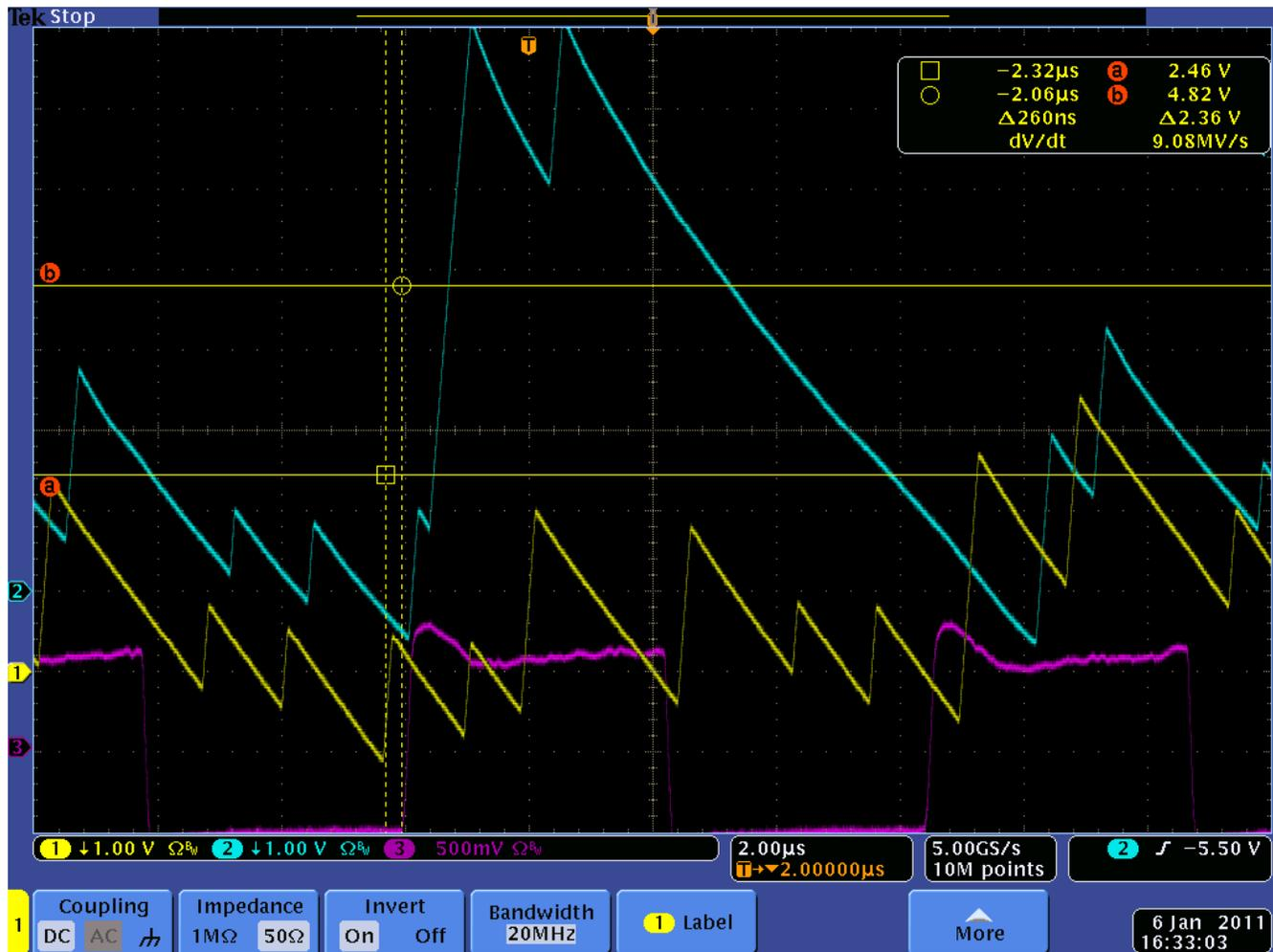
**Figure 3. Multiphase Regulator Phase Imbalance During a Load Transient – No Ripple Cancellation.**
