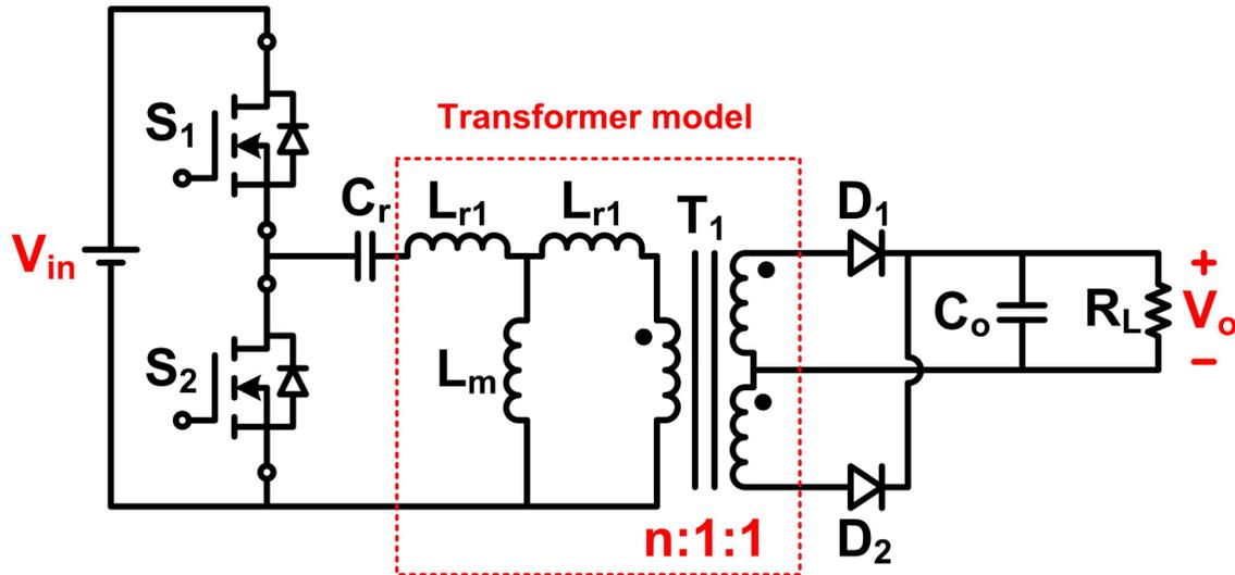
Figure 2. Isolated LLC Series Resonant Converter with Integrated Transformer
