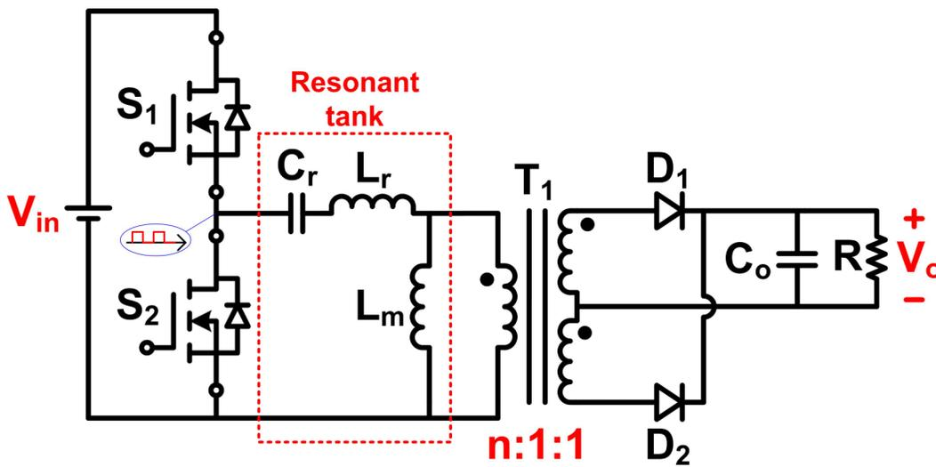
**Figure 1. Basic Isolated LLC Series Resonant Converter**
