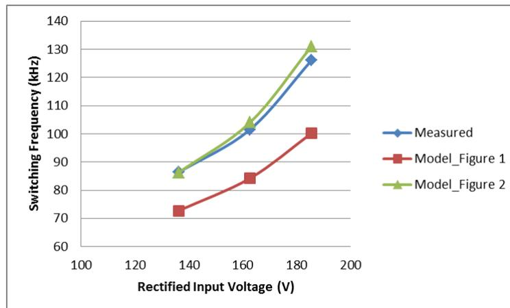
Figure 3. Comparison between Calculated and Measured Switching Frequencies of PMP8762
