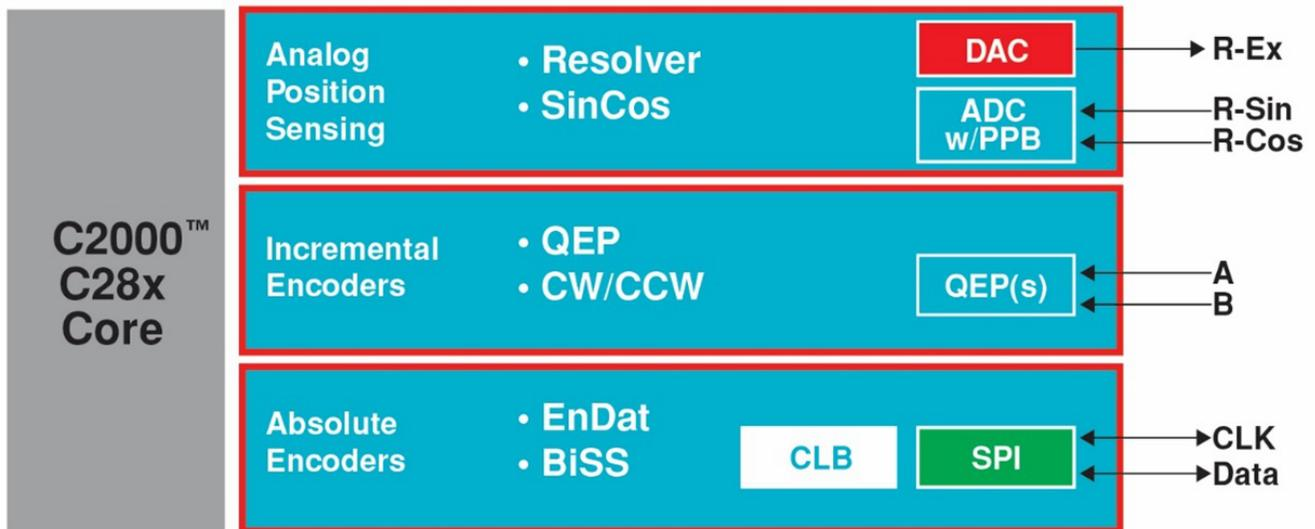
The F28379 MCUs are the first commercial microcontrollers offering the breadth of position sensor support, flexibility, scalability and robustness to make the need for custom FPGA support a thing of the past. Solutions for these four sensors as well as incremental encoders are included at no charge as part of the controlSUITE™ software suite.
