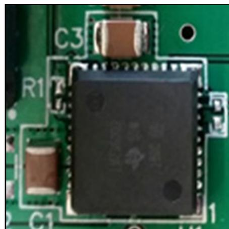
Figure 2. 60V 2A power-module solution
