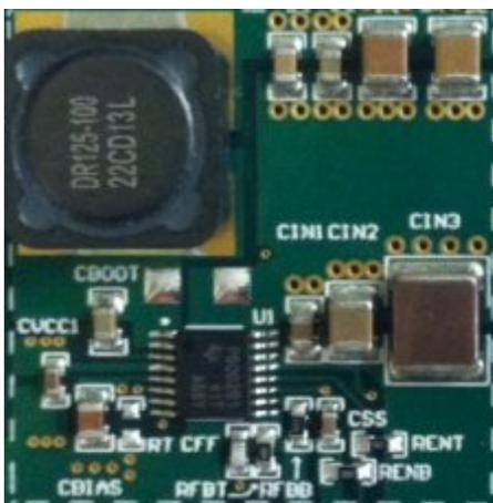
Figure 1. 60V 2A discrete solution
