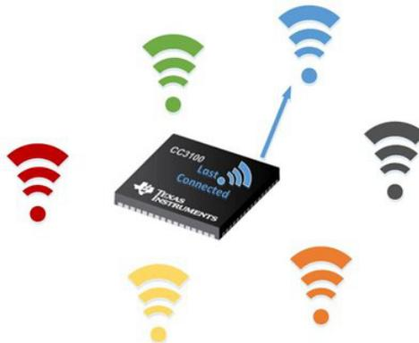
**Fast connect** – This feature configures the device to connect to the last access point (AP) that it was connected to instead of performing a scan (searching for APs). Eliminating the need for a scan reduces the device's energy consumption. Fast Connect can be configured using the [“CC3100\\_sl\\_WlanPolicySet”](#) & [“CC3200\\_sl\\_WlanPolicySet”](#) APIs.
