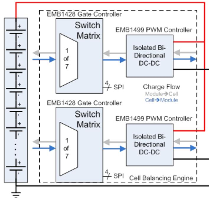
**Figure 2. TI Designs (TIDU239) EM1401EVM Simplified Architecture**
