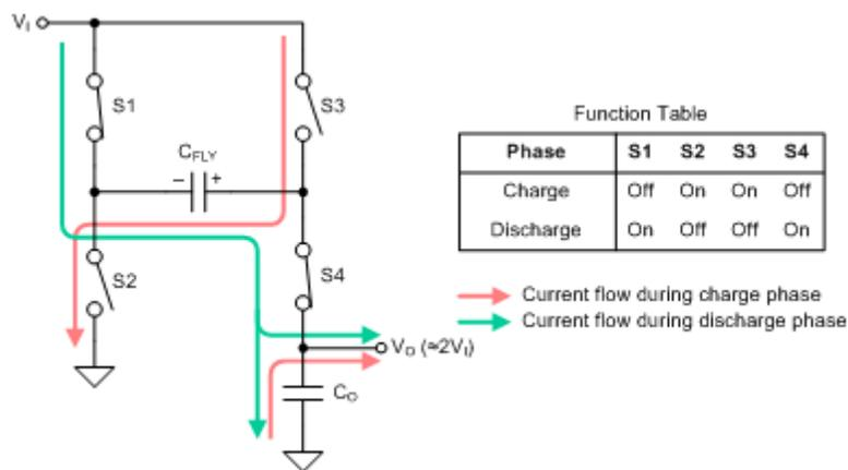
**Figure 1. Simplified Charge-pump Block Diagram (Voltage Doubler)**
