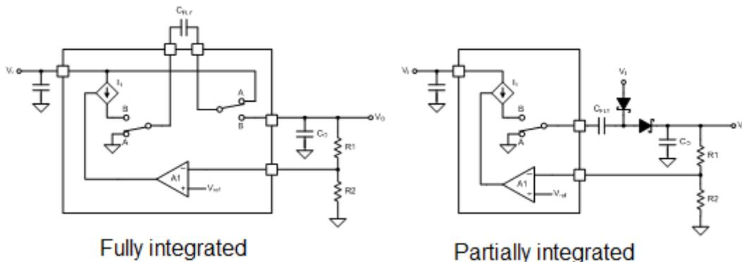
**Figure 3. Different Charge-pump Integration Levels**
