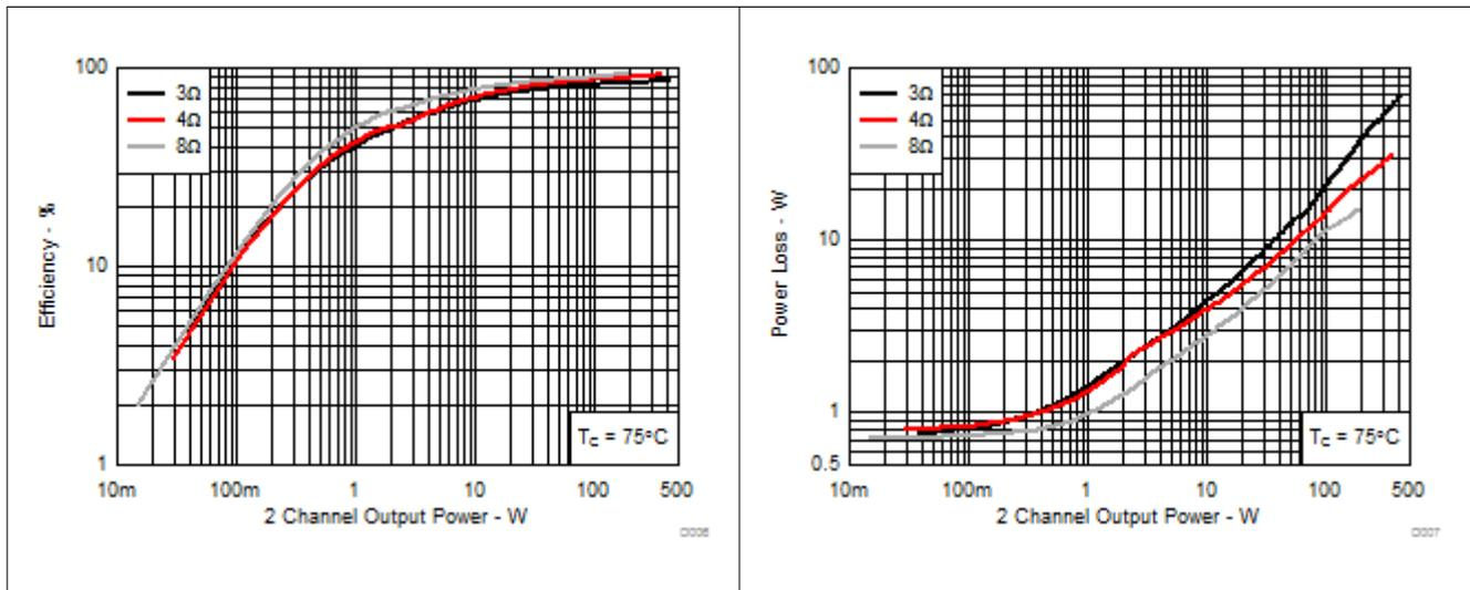
**Figure 1. Example of TPA3251 Power Efficiency and Power Loss vs. Output Power**
