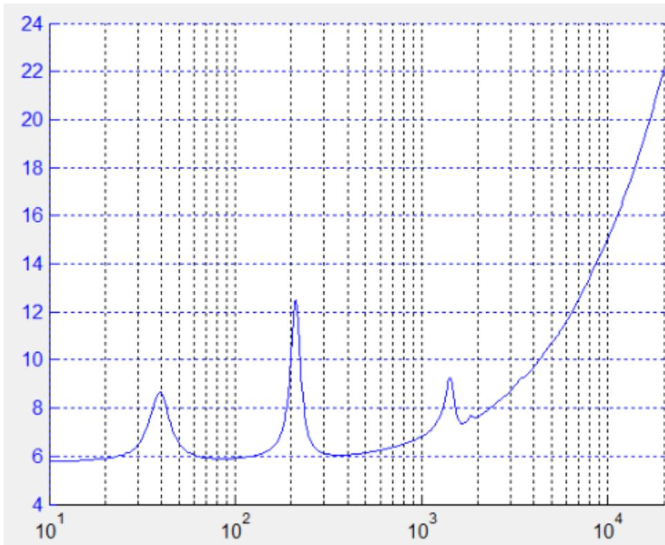
**Figure 3. Example Loudspeaker Impedance (Vented Box)**
