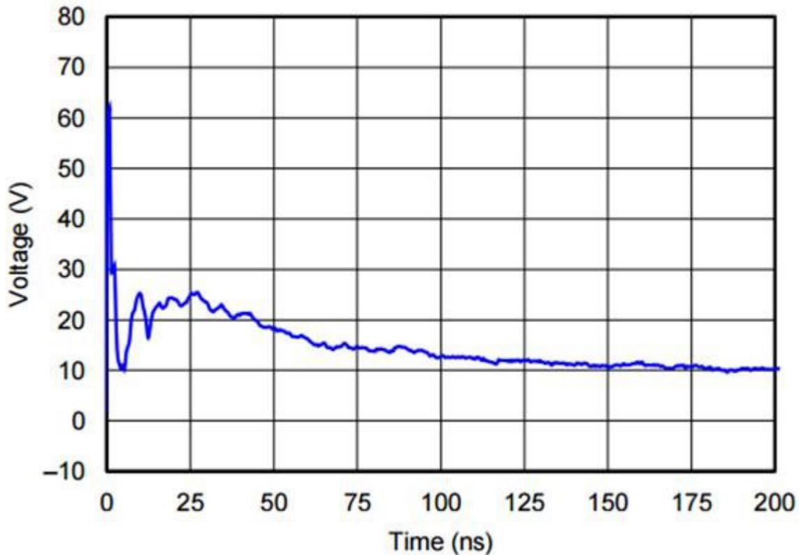
**Figure 2. TPD4E05U06 IEC 61000-4-2 Clamping Voltage, +8kV Contact**
