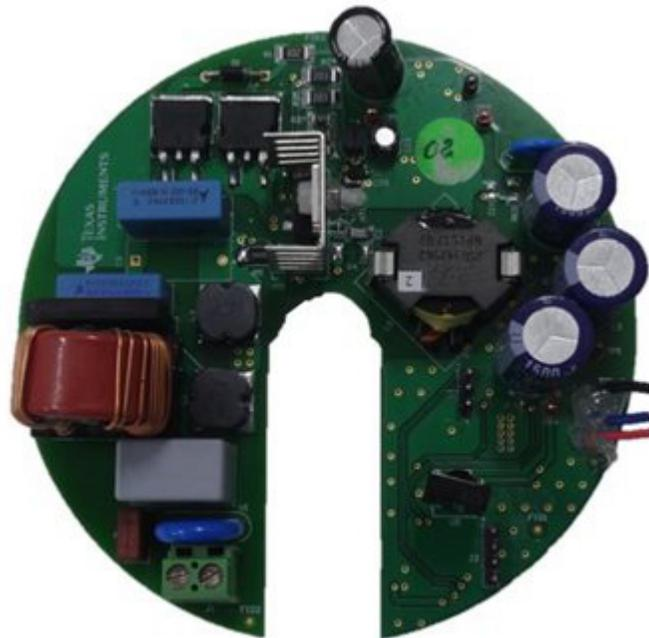
**Figure 1. Board Image of TI Design: Mains-operated, 24V, 30W BLDC Motor Drive W/highly Efficient, High Power Factor Power Supply (TIDA-00652)**
