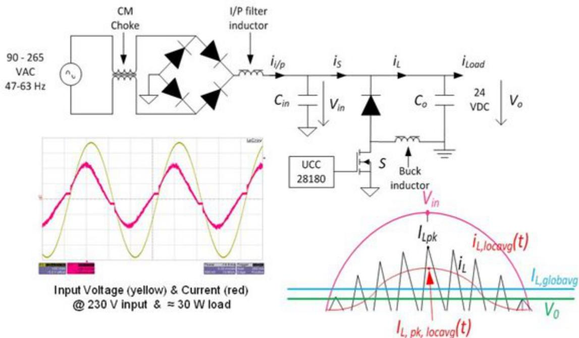
**Figure 3. Circuit Diagram of the Buck PFC Topology**
