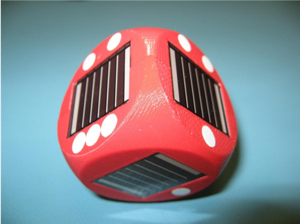
**Figure 1. The Solar Dice Is an Example of an IoT Sensor Node**
