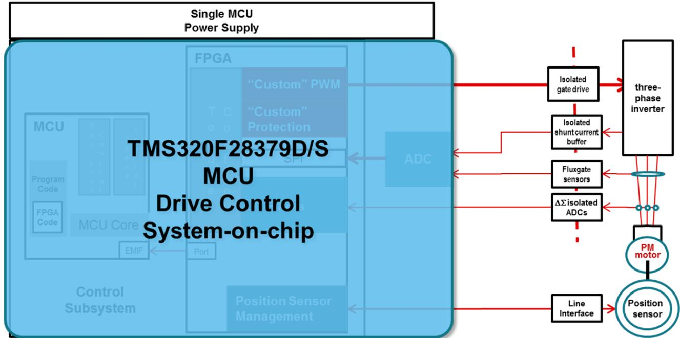
Figure 2. Industrial drive control SoC-- C2000 TMS320F28379 MCU
