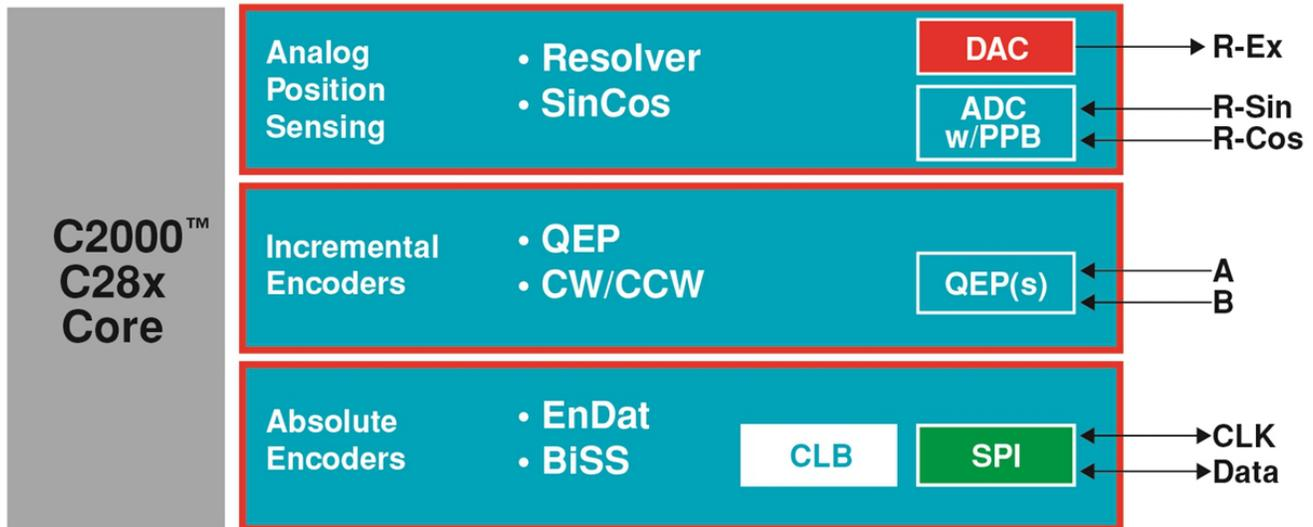
Figure 3. Leading analog and digital position sensors supported
