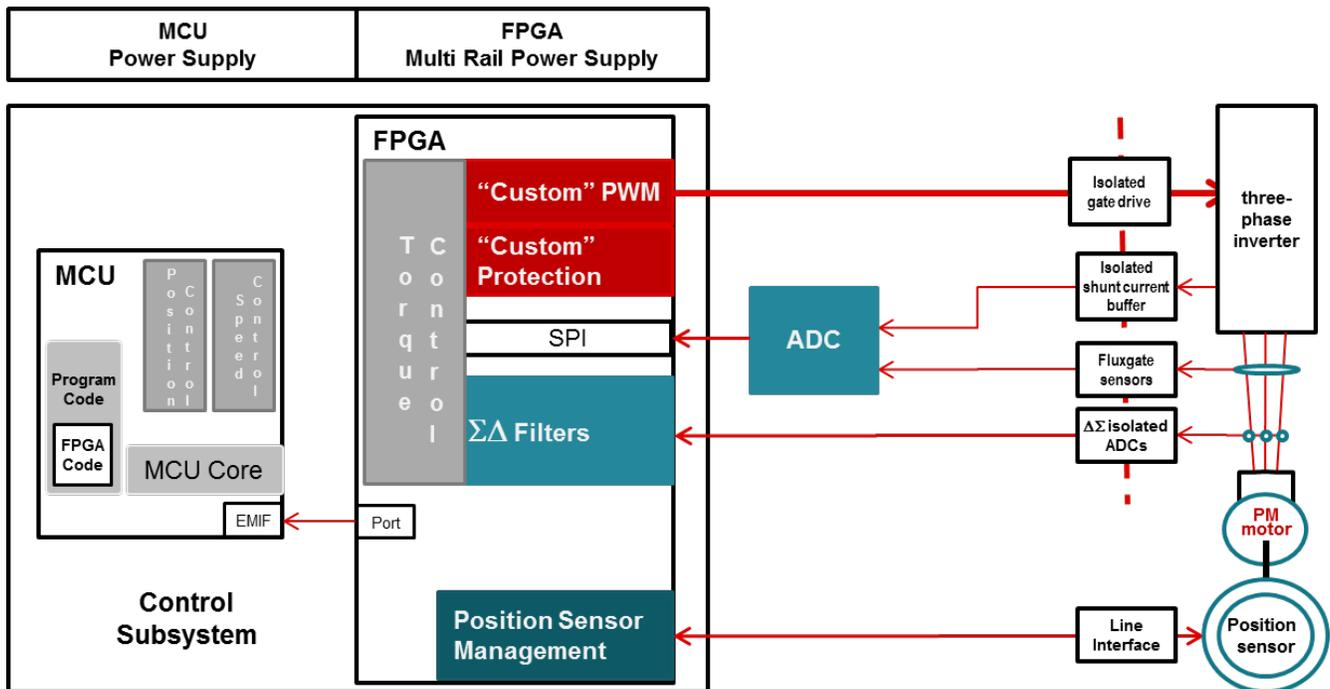
Figure 1. Industrial drive system, MCU + FPGA
