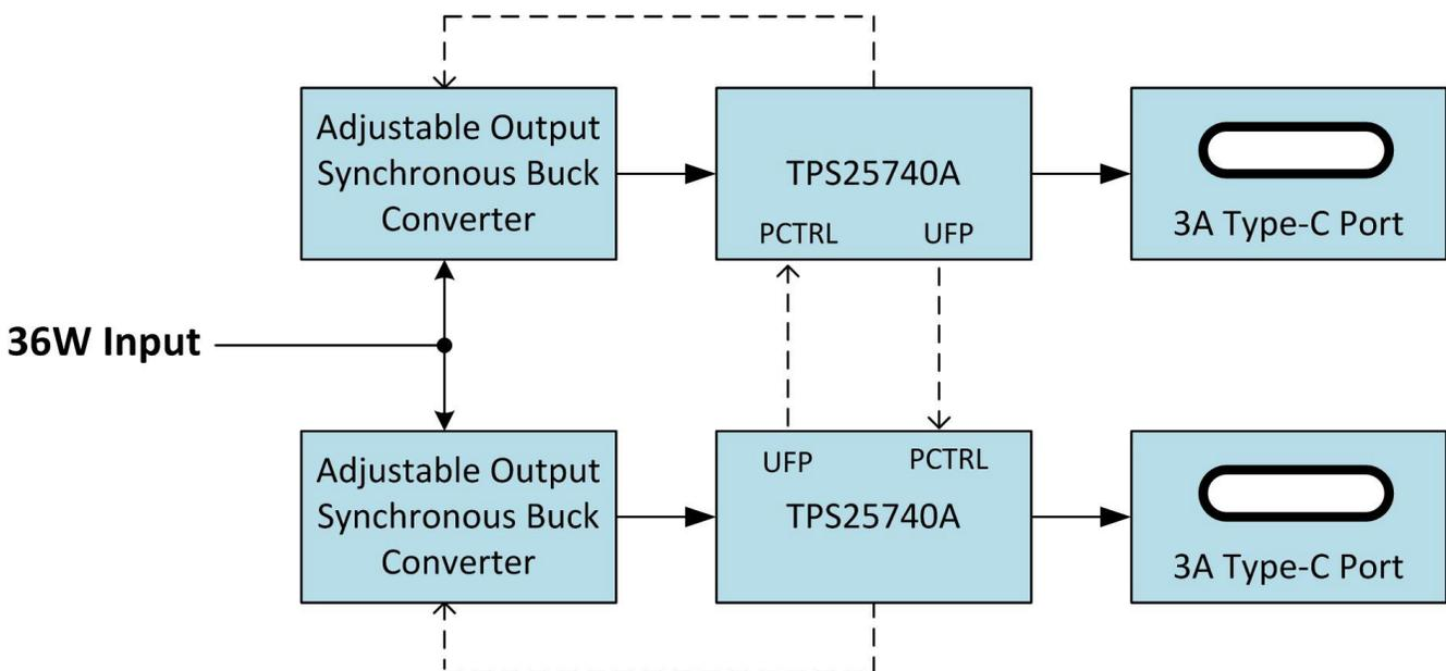
**Figure 1. This 36W System with Port Power Management Intelligently Shares Power between Two Ports**
