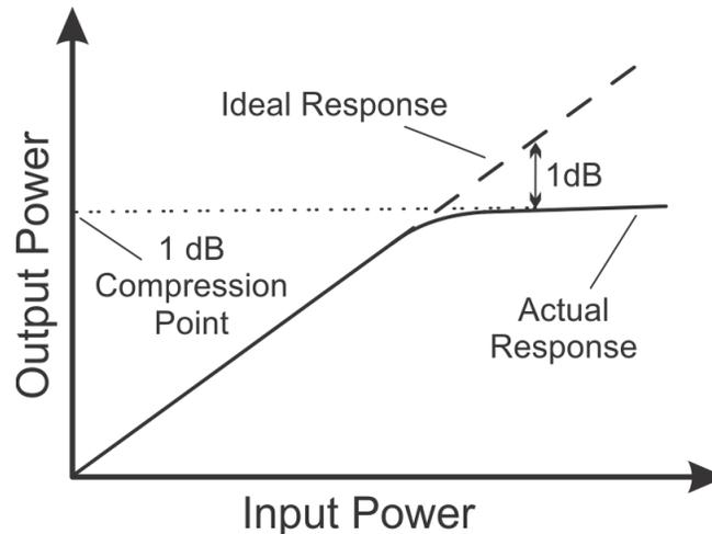
**Figure 2. Output P1dB Example**
