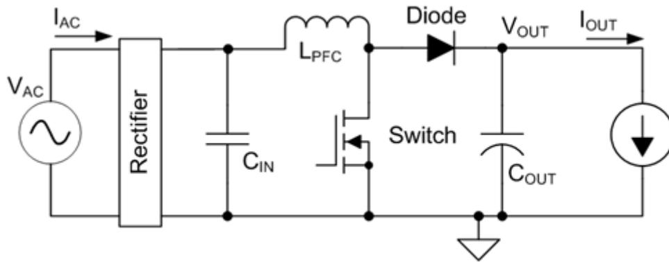
**Figure 1. Typical Boost PFC Schematic**
