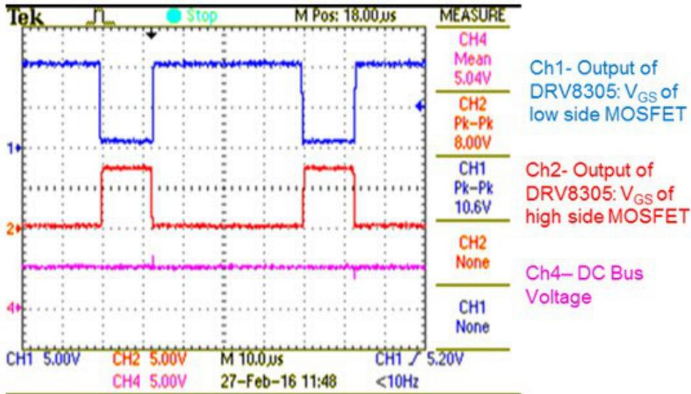
**Figure 3: Low- and high-side gate-drive output from the DRV8305 at a DC input voltage of 5V**
