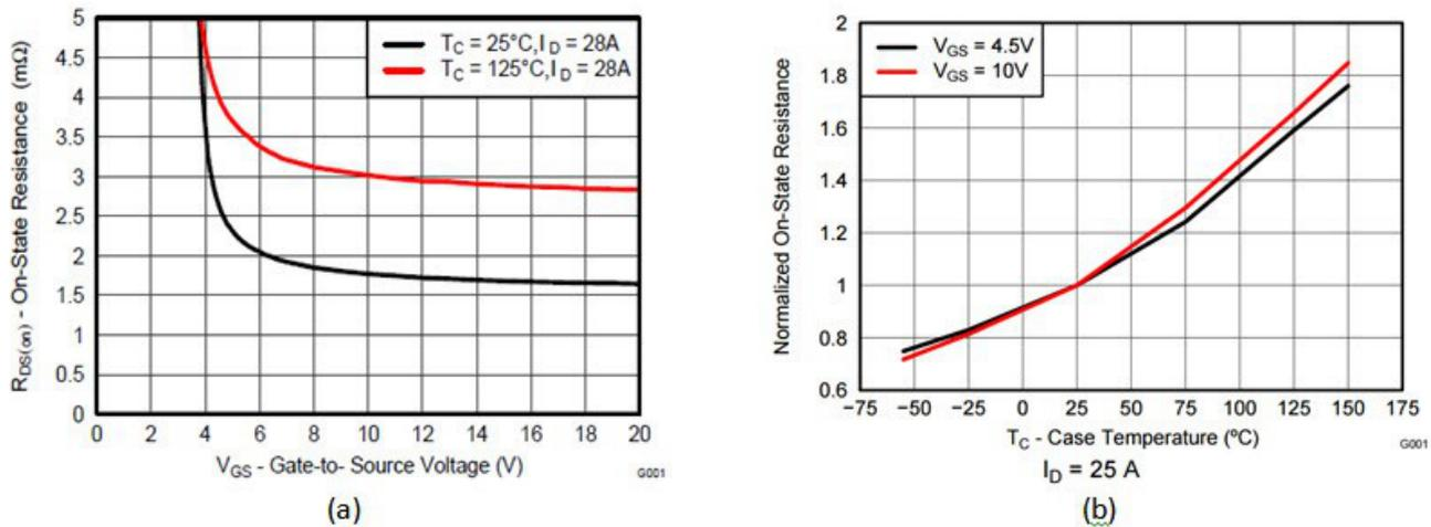
**Figure 1: Variation of  $R_{DS\_ON}$  with  $V_{GS}$  (a); and with temperature (b)**
