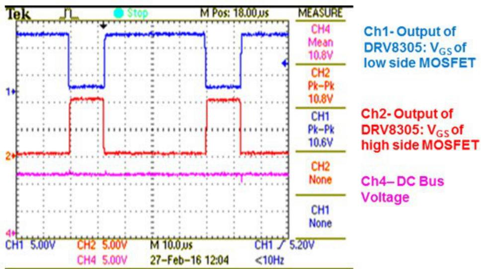
**Figure 2: Low- and high-side gate-drive output from the DRV8305 at a DC input voltage of 10.8V**
