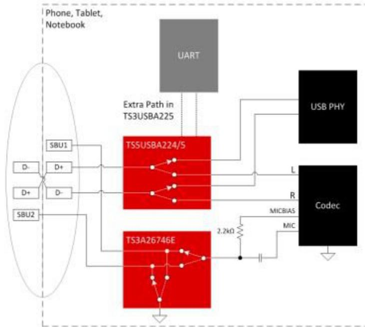
**Figure 2. Analog Audio Signal Routing from USB Type-C Connector**
