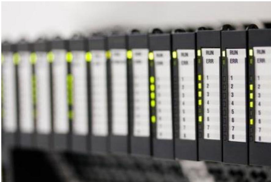
**Figure 1. PLC I/O Module Array**
