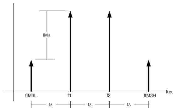
**Figure 2. Frequency Representation of Third-order Intermodulation Distortion**
