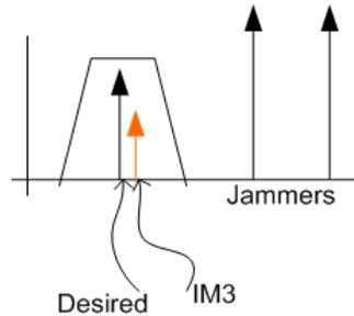
**Figure 3. IM3 Desensitizing a Receiver**
