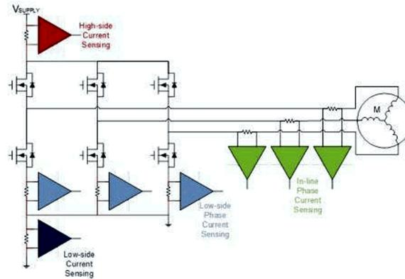
**Figure 2. Circuit Diagram Showing Four Potential Current-measurement Options for Three-phase Motor Implementations**
