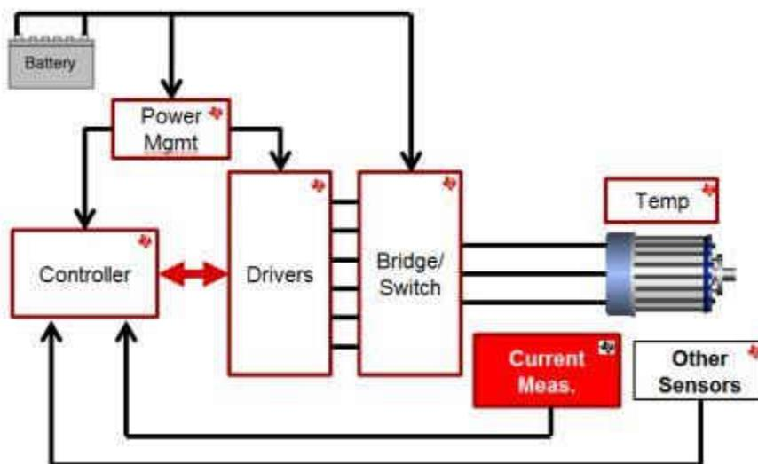
Figure 1. A Typical EPS System
